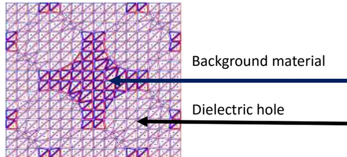
Figure 1. The cross section of PCF and the mesh
